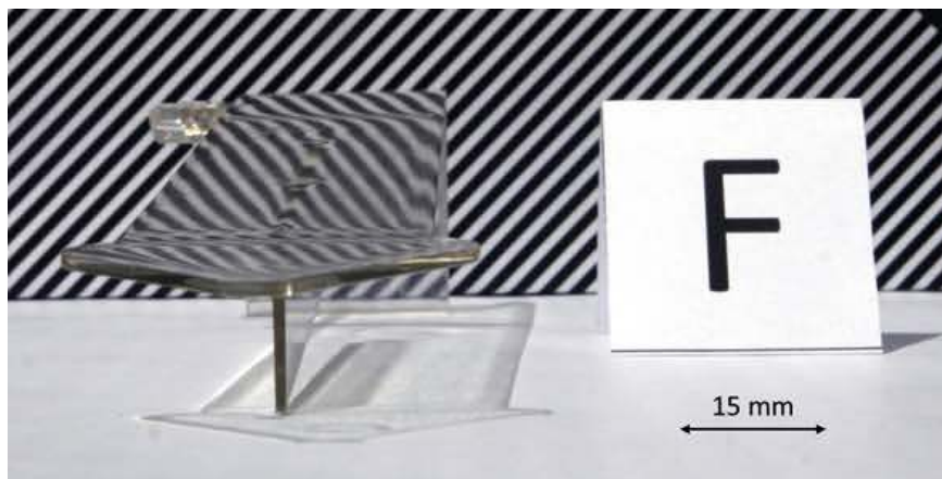
Fig. 3. Using a striped pattern, sink marks on the part surface can be detected
