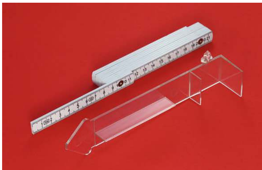
Fig. 2. The test part was produced with different thickness and two different injection points
