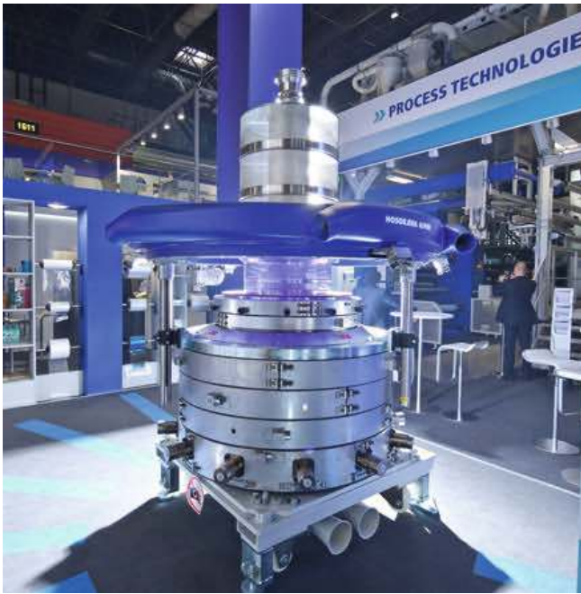
Fig. 2. Eleven-layer die-head from the X-series (figure: Hosokawa Alpine)
