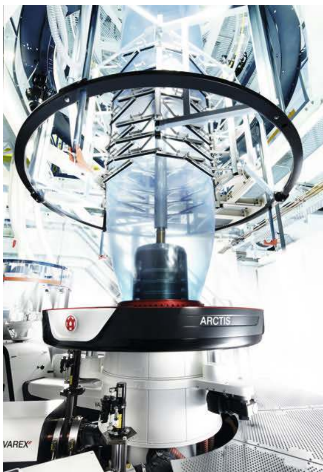
Fig. 1. The air ring of the Varex II blown-film line is made of GRP (figure: Windmüller & Hölscher)
