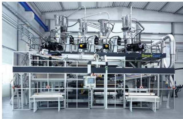
Fig. 9. The Smart Cast system for stretch films can produce film at a rate of up to 1.5 t/h in a thickness of 12 µm (figure: SML)
