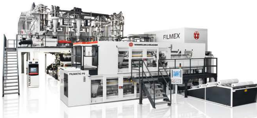
Fig. 10. Filmex cast film line with nano-layer feed block for the production of stretch film (figure: Windmüller & Hölscher)
