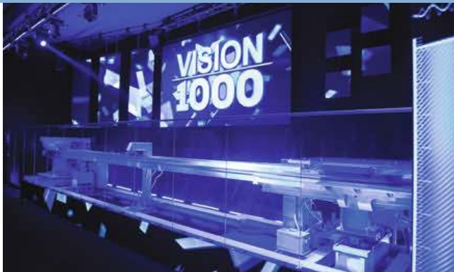
Fig. 12. This chain guide capable of 1,088 m/min is the first step toward achieving the stated production goal of 1,000 m/min (figure: Brückner)
