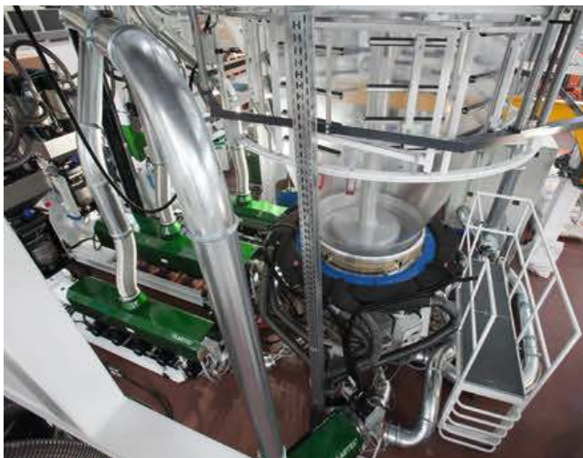
Fig. 5. The CR-K3 air ring of carbon fiber-reinforced plastic improves air flow and increases productivity (figure: Macchi)
