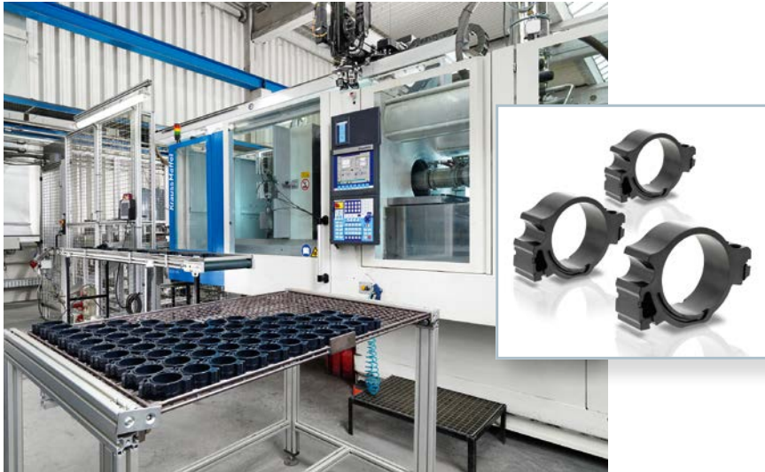
Fig. 1. Precision parts with only 10 \mu\text{m} tolerance: the oil pump adjusting ring of PF (MD+GF) 70. Production has been running since 2014 in continuous three-shift operation on a CX200 © KraussMaffei)
