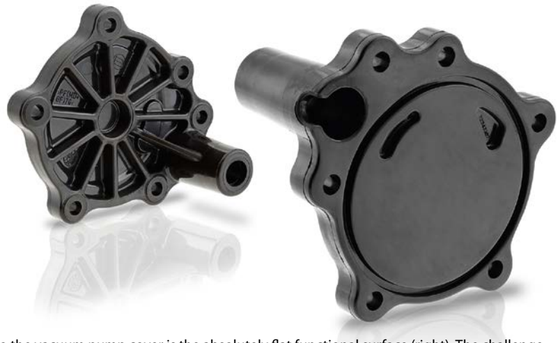
Key to the vacuum pump cover is the absolutely flat functional surface (right). The challenge here is that the pronounced rib structure on the reverse side (left) must not show through on the flat side. This can be solved by using PF thermoset compounds (© KraussMaffei)
