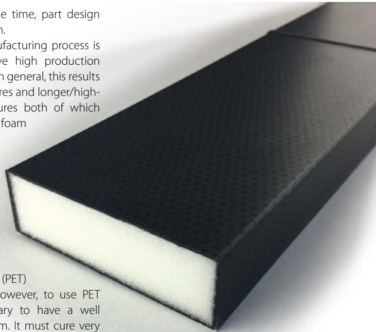
Good surface quality, pristine foam core: a cross-section through an HP-RTM part with carbon-fiber reinforcement of Airex T10.110 core and Henkel Loctite Max 2 PU resin
