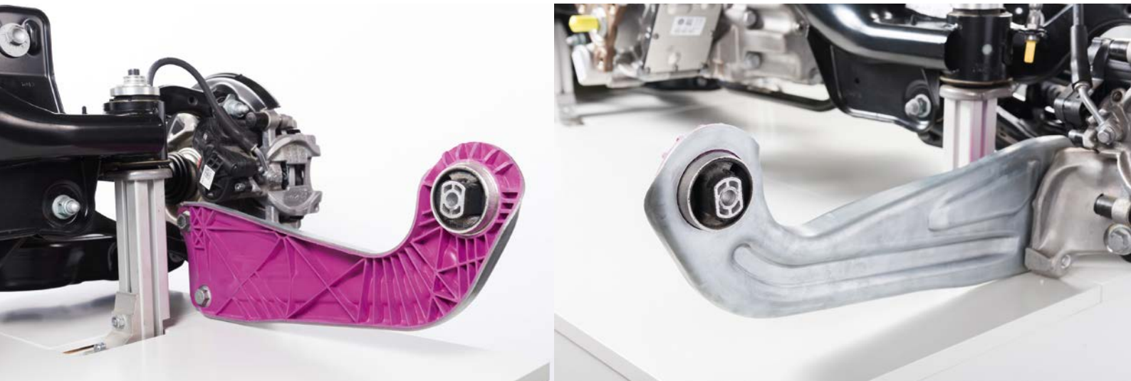
The longitudinal control arm of a rear suspension system made from a hybrid comprising long fiber-reinforced PA6 and steel sheet is formed and bonded in one step. The two materials combine lightweight design with fail-safe crash behavior (© Evonik)
