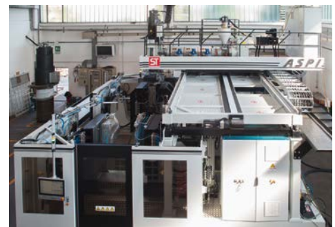
ST Aspi 150.3 Duo: the machine can handle two different recipes at the same time (© ST Blowmoulding)
