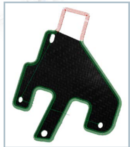
Fig. 2. Typical measurement of the contour of an organic sheet with a camera system reveals possible defects (shown in red) (© KraussMaffei)
