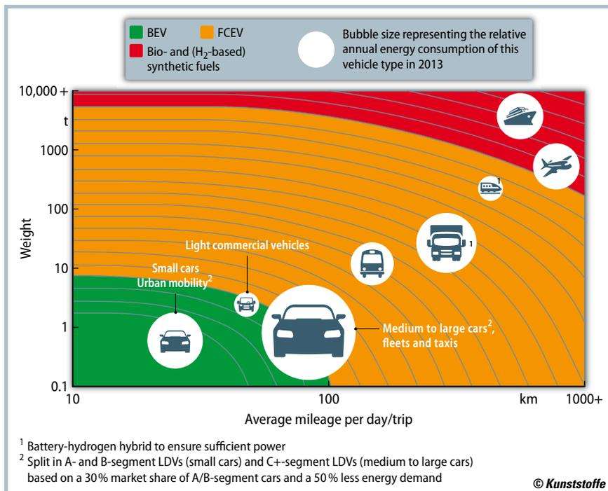
Fig. 2. Current and future application fields of fuel cells in the transport sector [4] BEV: battery electric vehicles; FCEV: fuel cell electric vehicles (source: Hydrogen Council)
