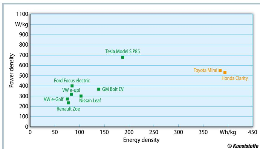
Fig. 3. Comparison of commercial automotive battery (green) and fuel cell systems (orange), incl. hydrogen stores with 5.7 wt. % H<sub>2</sub> acc. to [5] (source: ETI Group)
