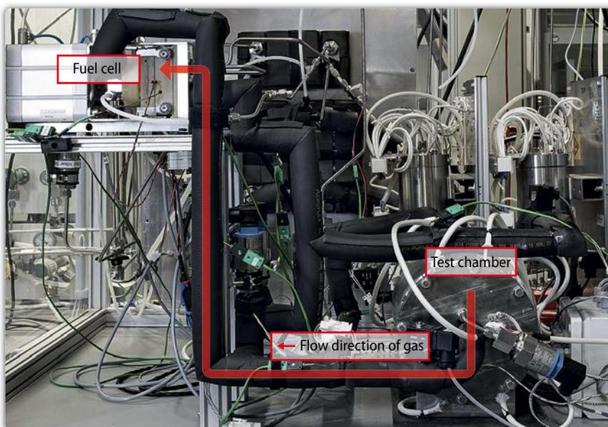
Fig. 6. Set-up for investigating material samples for fuel cell suitability (source: ZBT, A. Kayser)
