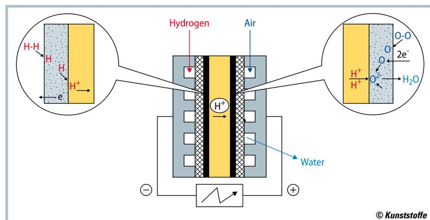
Fig. 4. Schematic view of the construction and the electrochemical reactions of a membrane fuel cell (source: A. Heinzel)
