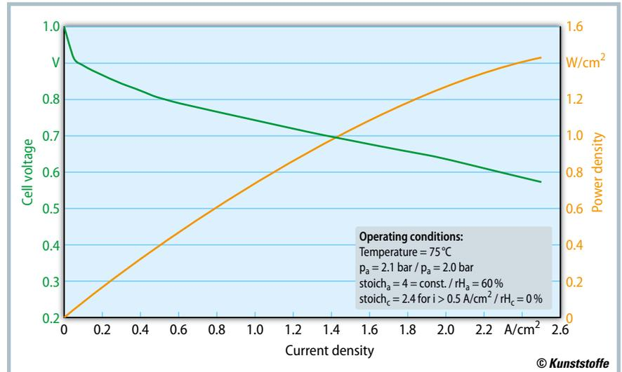
Fig. 5. Current density-voltage curve of a PEM fuel cell (source: ZBT, Dr. Jörg Karstedt)
