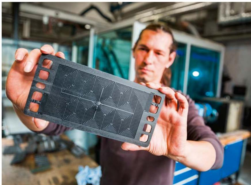
Injection-molded bipolar plate of plastic-carbon compound (© JRF e.V.)
