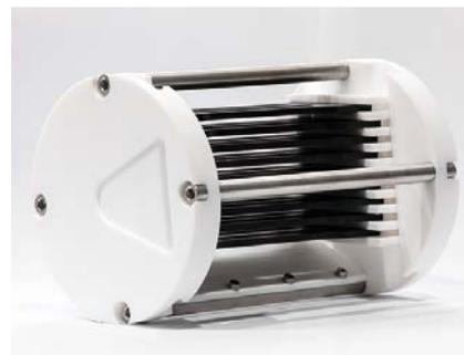
**Fig. 7.** Test rack within the test chamber with the possibility of positioning a total of 27 material samples (© ZBT, A. Kayser)
