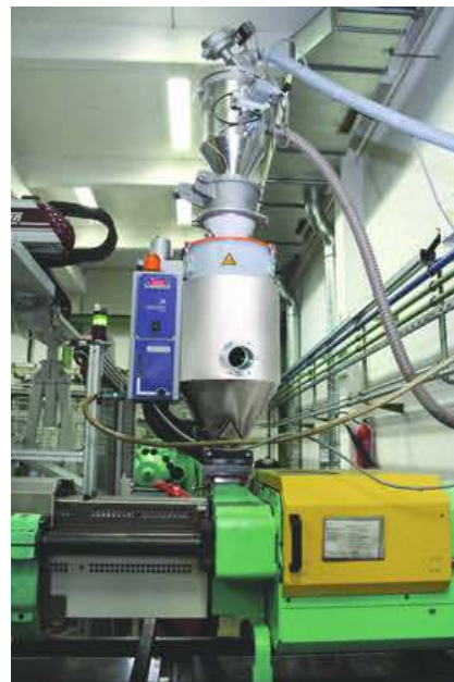
Fig. 6. For safety sake, Hillers is installed machine-mounted dryers that can be used as necessary to prevent renewed uptake of moisture by the material pellets on the machine
