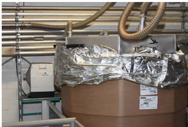
Fig. 5. To address renewed uptake of moisture by the material in the octabin, the container is covered. In addition, its content is maintained under a permanent blanket of dry air
