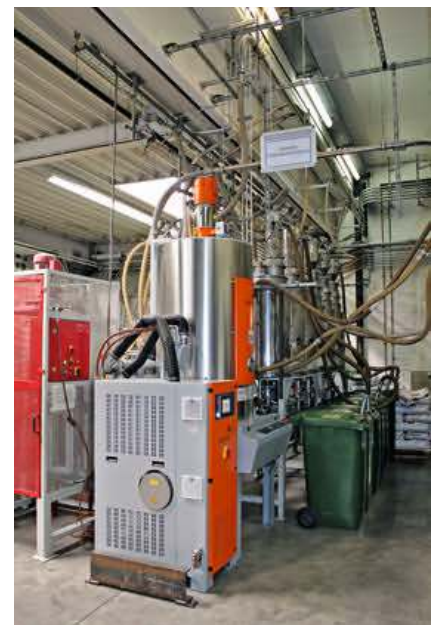
Fig. 4. Fitted with automatic temperature and dew point leveling (ATTN), the Luxor A 120 dry air generator controls the dew point of the process supply air with an accuracy of ±1°C
