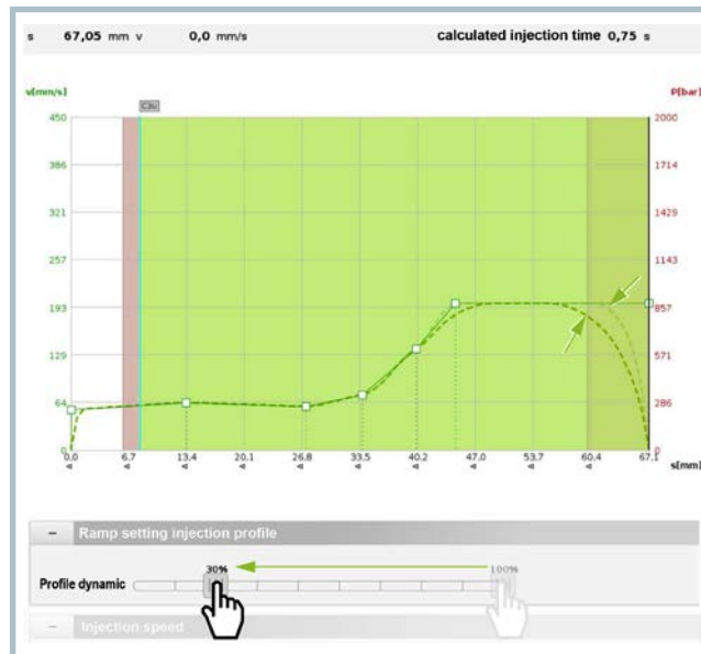
Fig. 1. The precalculated speed profile (broken line) shows the expected speed profile based on the set setpoint values. By changing the profile dynamics, the movement can be made more gentle or more dynamic. The effect is visible directly during the movement of the slider (© Engel)
