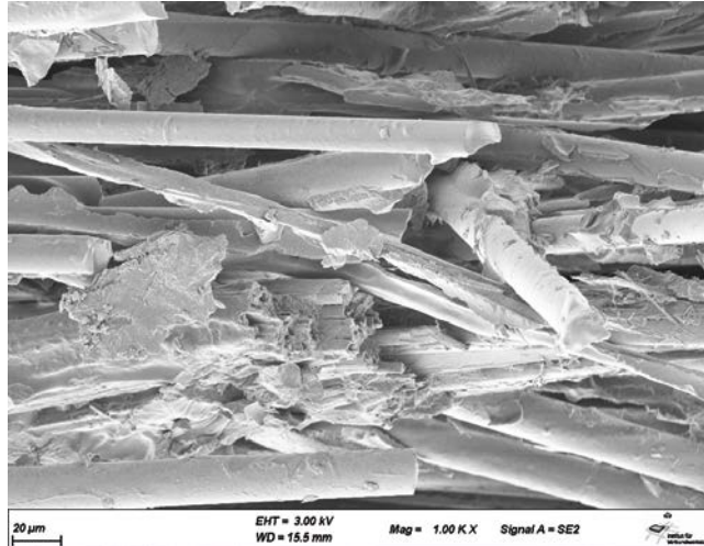
Fig. 6. The scanning electron micrograph of the fracture surface of the acrylic-NF/BF composite shows a homogeneous fracture surface without individually pulled-out fibers
