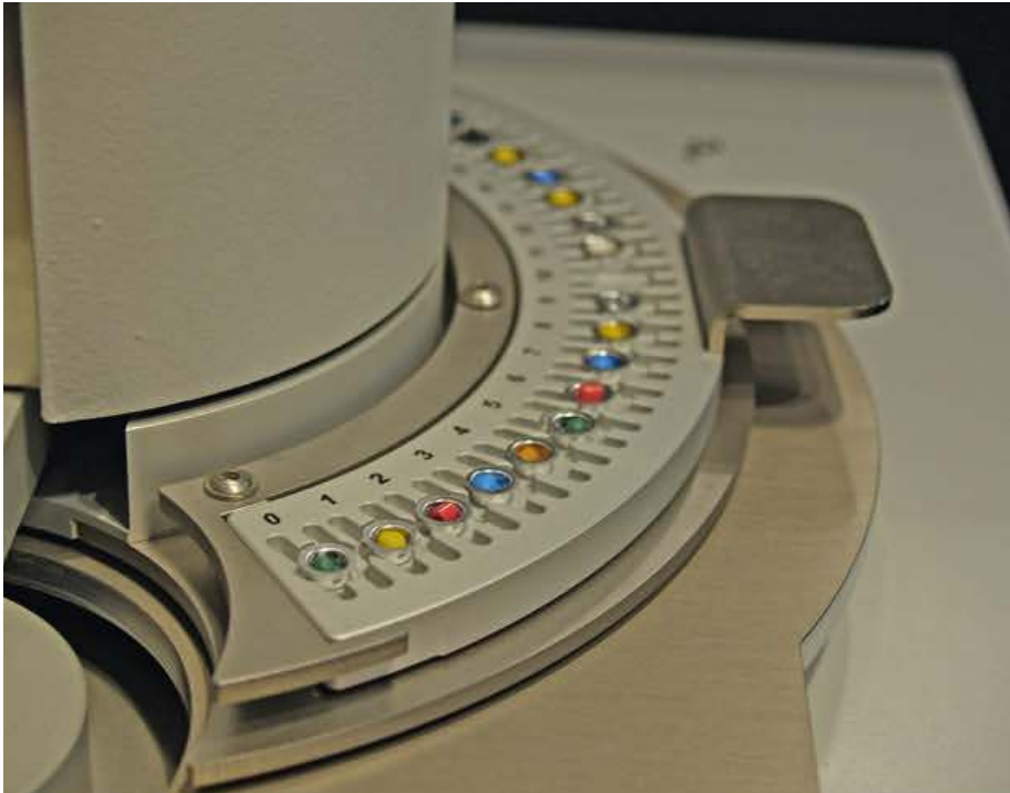
Fig. 4. Samples prepared for differential scanning calorimetry. The pellets must be manually disintegrated previously, filled into crucibles and placed on the instrument. From then on, the measurement runs fully automatically
