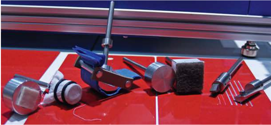
Fig. 1. For many companies, the automotive industry is and will remain an innovation driver. The test head for textile abrasion on plastic materials (3rd from left) was developed together with users (figures: F. Gründel)
