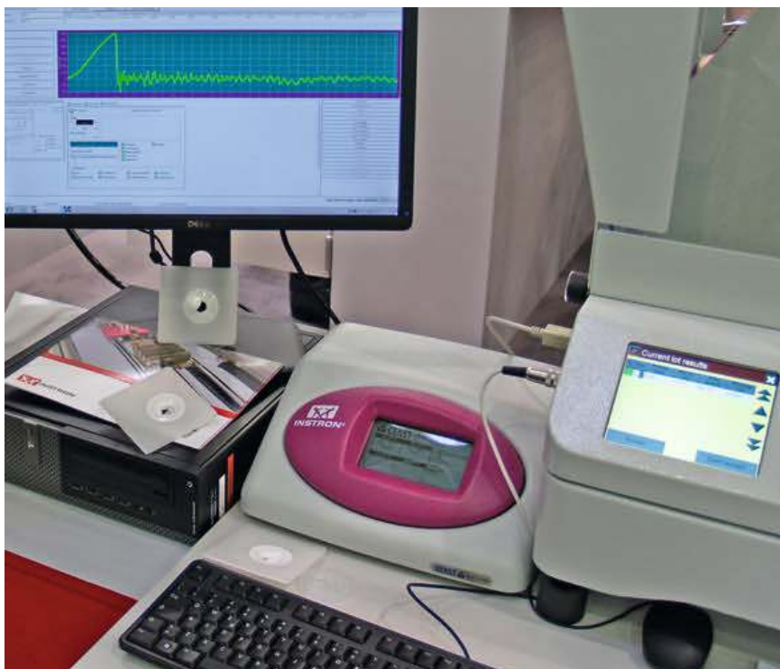
Fig. 2. High-speed data acquisition is interposed between the test instrument and computer evaluation. Here, a high measurement rate is required in events such as pendulum machines and drop towers
