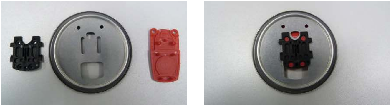
Fig. 2. The four small pin domes are quickly riveted leak-tight in the first process step. Left: inner and outer slide before ultrasonic riveting, right: riveted parts
