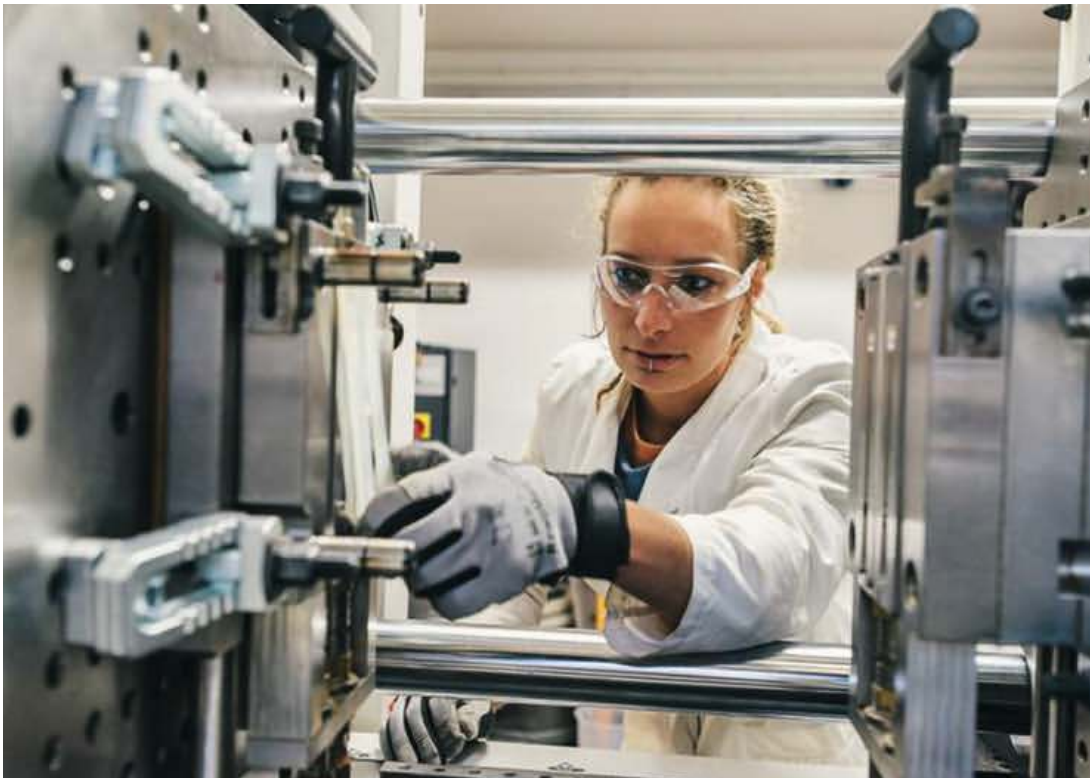
Bioplastics such as polylactide can be injection molded to yield on-spec articles
