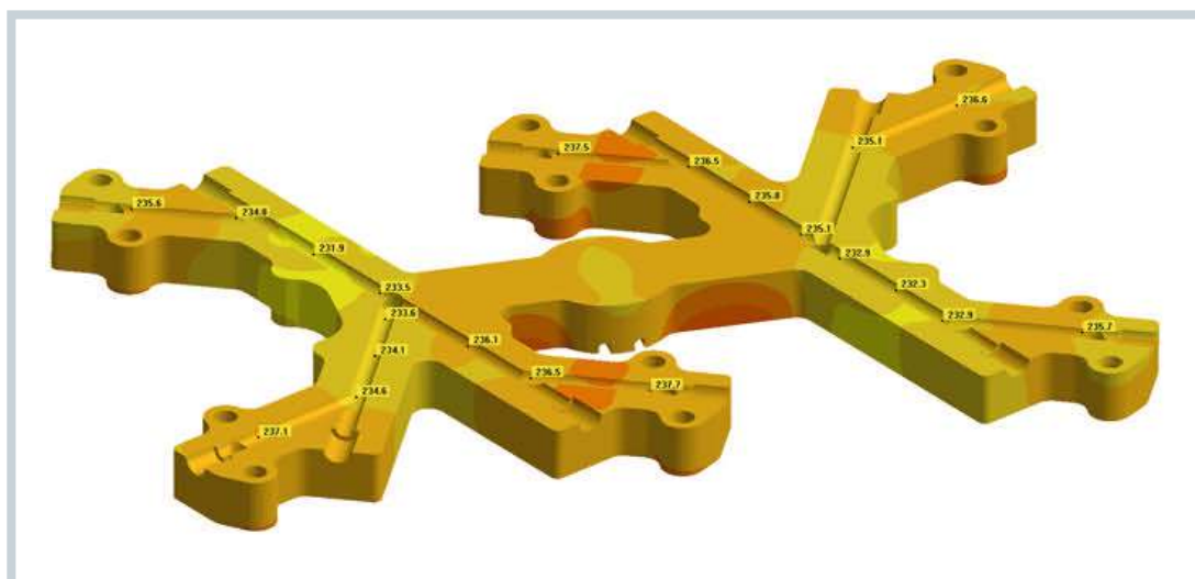
Fig. 1. Molds tailored rheologically, thermally and mechanically to their application ensure high parts quality and productivity
