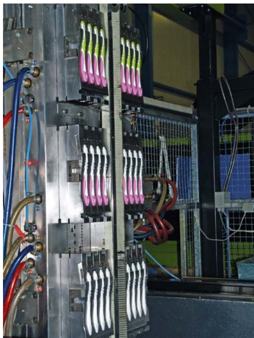
Flexible but not fast: in a 3x8-cavity platform mold with transfer technology, straight 3-component handles for toothbrushes are produced (figure: Doriat)
