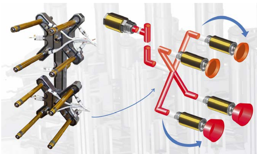
Fig. 3. Potential scenario in the 8-fold hot runner system: as a result of distributing the melt flow with an asymmetrical shear profile, branches form in the manifold with different levels of viscosity – the outer cavities are thus filled first in this instance; orange: lower shear, red: higher shear
