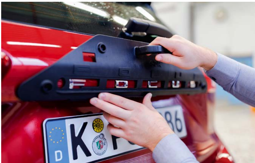
For the precise placement of logos, branding marks and vehicle lettering Ford also uses additive templates and jigs in series production © Ultimaker
