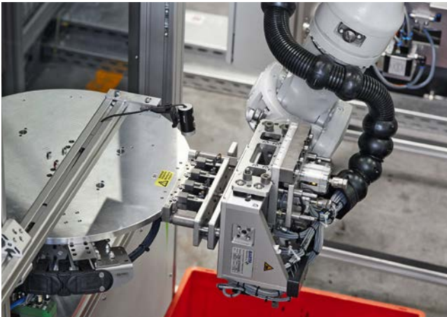
The second robot receives the four inserts and eight contacts from the feed cell (left) and also places them in the injection mold (right)
