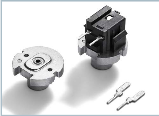
The connector carrier for the stop/start system consists of a metal insert and plug contacts, which are fed correctly positioned at two stations and then overmolded with glass-fiber-reinforced PBT
