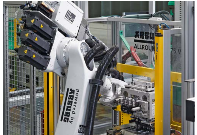
The second robot receives the four inserts and eight contacts from the feed cell (left) and also places them in the injection mold (right)
