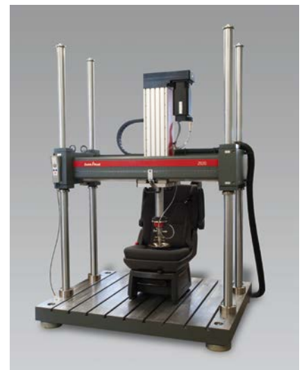
A new test stand is ideal for fatigue testing of foams (figure: Zwick)
