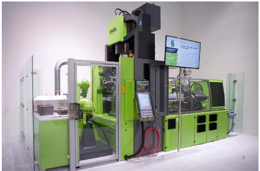
Fig. 2. Compact Engel manufacturing cell for processing thermoplastic FRP. The IR heating station for heating organic sheets is integrated into the cell (rear left in the figure), and operates completely controlled and quality monitored (figure: Engel)
