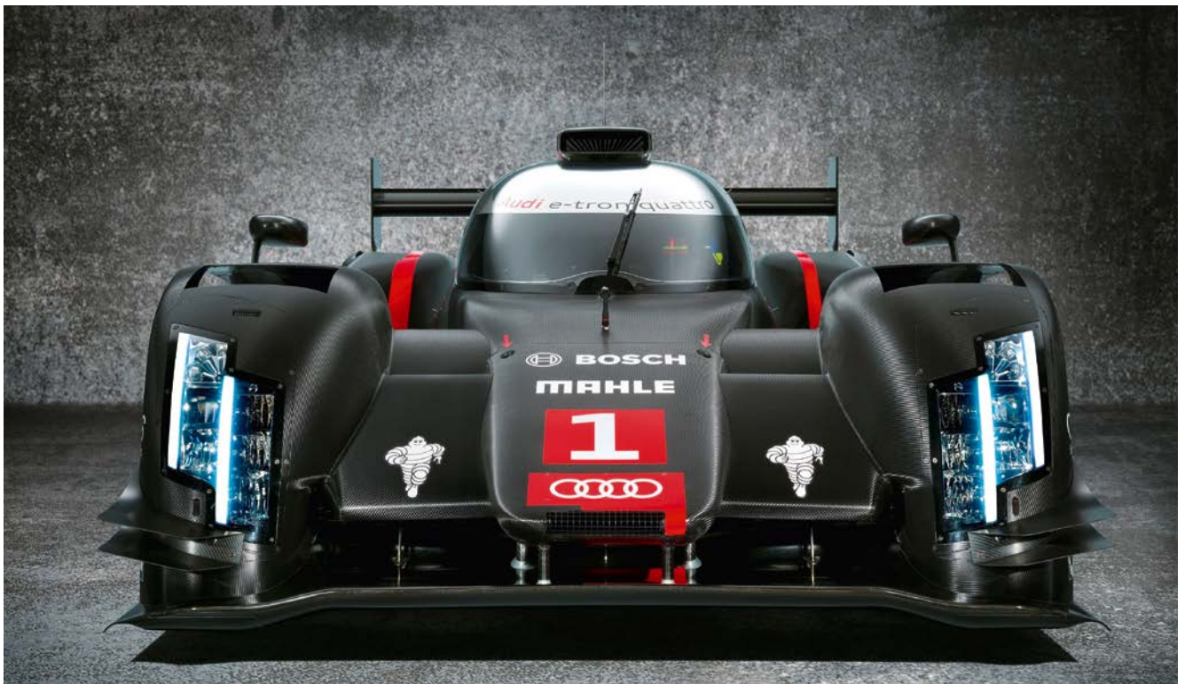
Racing as example: Fiber-reinforced plastic composites make the Audi R18 e-tron quattro extremely lightweight (figure: Audi)
