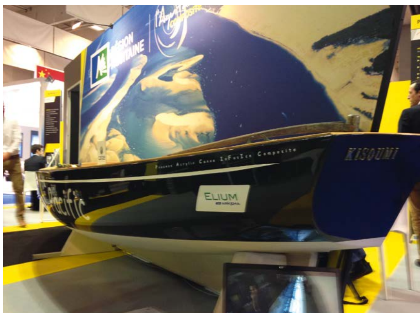
Fig. 3. In-situ acrylate enables infusion at ambient temperature and yields damage-resistant components: CFRP boat with a thermoplastic matrix (figure: Arkema/Canoe)
