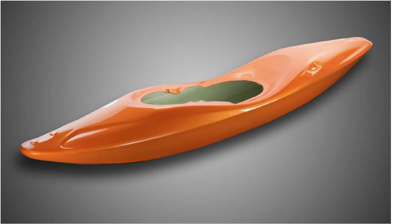
The fiber-reinforced polyamide kayak was designed by Haluzka. It was produced by in-situ polymerization in a vacuum infusion process (figure: BASF)
