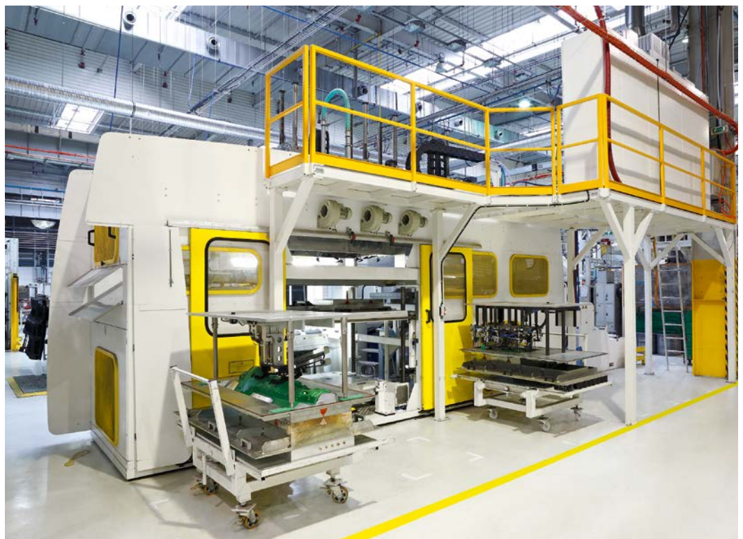
Example of a in-line vacuum laminating machine (figures: Frimo)
