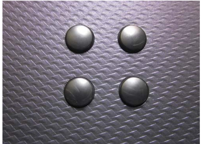
Fig. 4. Socalled pads integrated with the IMG process
