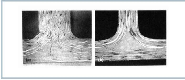
**Fig. 5.** Undulations in a stringer foot
