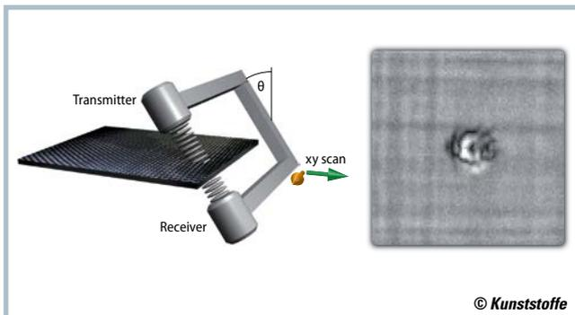
Fig. 11. Air-coupling ultrasound scan in transmission mode and measurement result
