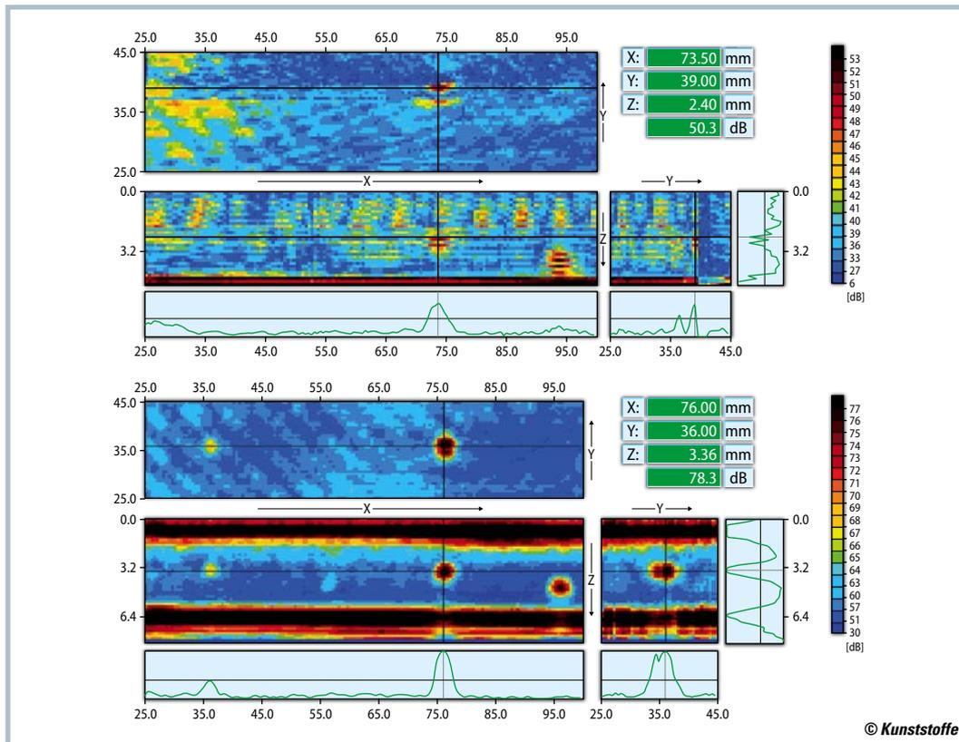
**Fig. 9.** Top: C scan and B scan by means of a conventional transducer; bottom: Matrix Array
