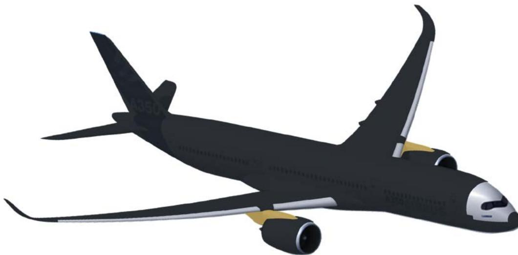
**Fig. 1.** Parts of the outer skin of the A350 are made of fiber-plastic composites (gray)
