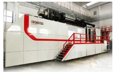
The third BI-Power 7000 tonne features a special twin barrel injection unit and co-injection nozzle, allowing a maximum shot size of 149 kg of PS (figure: Negri Bossi)
