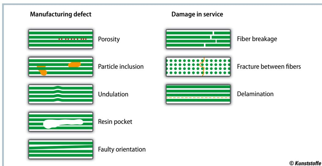
**Fig. 4.** Defects in fiber-plastic composites – during manufacturing and during service
