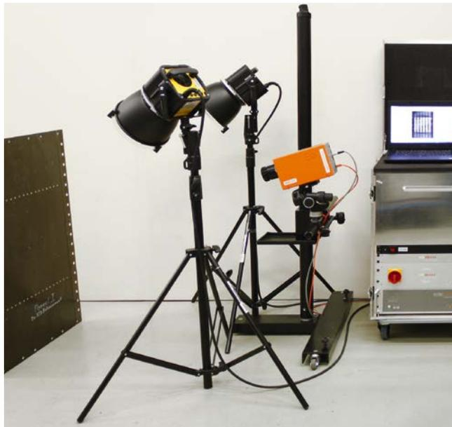
**Fig. 7.** Measurement set-up of thermography with optical excitation
