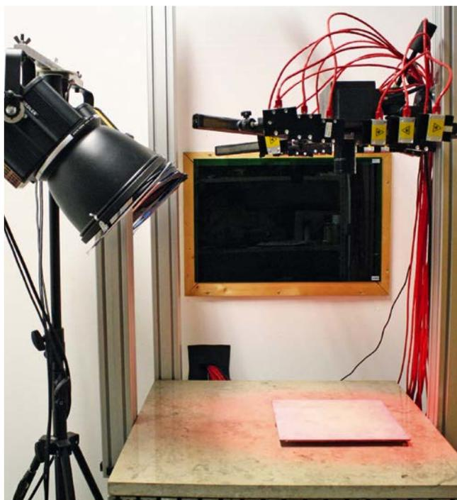
**Fig. 8.** Measurement set-up of shearography with optical excitation
