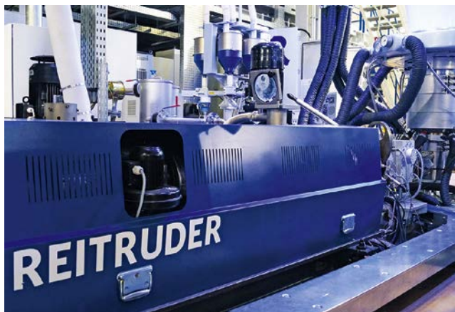
Fig. 1. REitruder (special co-rotating twin-screw extruder) installed in an Evolution 3-layer Blown Film Line (figure: Reifenhäuser)
