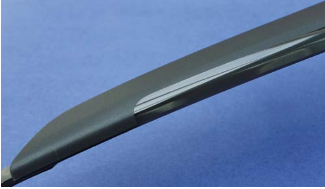
Fig. 7. Procedural in-mold assembly innovations allow absolutely seamless transitions from film surfaces to the plastics structures, even with variable insert thickness. The left figure shows the combination of a matte black décor film and a glossy molding surface, the right figure shows the seamless, gap-free embedding of a hard-coated clear-screen made of PC (figures: R. Bauer)
