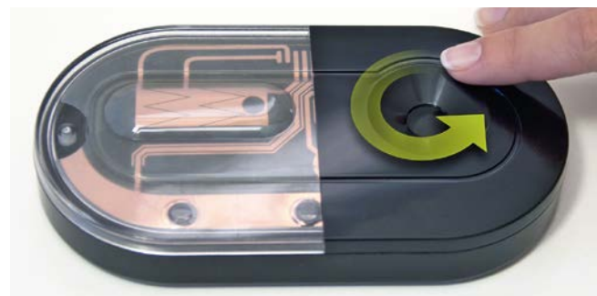
Fig. 1. The first “touchskin” demonstration object from 2010. The elementary functional unit is a back-molded film on the inner surface of the lid with printed-on electronic structures. The outer décor film includes the function-indications. Immersions in the cover function as finger guidance (figure: plastic electronic)
