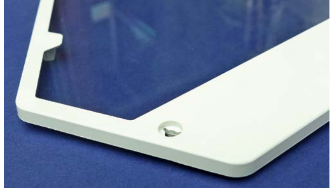
Fig. 7. Procedural in-mold assembly innovations allow absolutely seamless transitions from film surfaces to the plastics structures, even with variable insert thickness. The left figure shows the combination of a matte black décor film and a glossy molding surface, the right figure shows the seamless, gap-free embedding of a hard-coated clear-screen made of PC (figures: R. Bauer)
