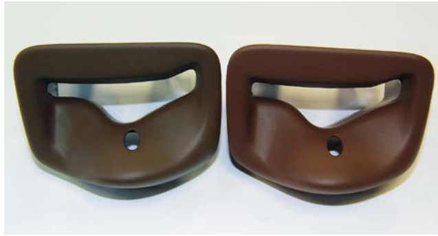
Fig. 1. Plastic components with (right) and without (left) a UV additive
