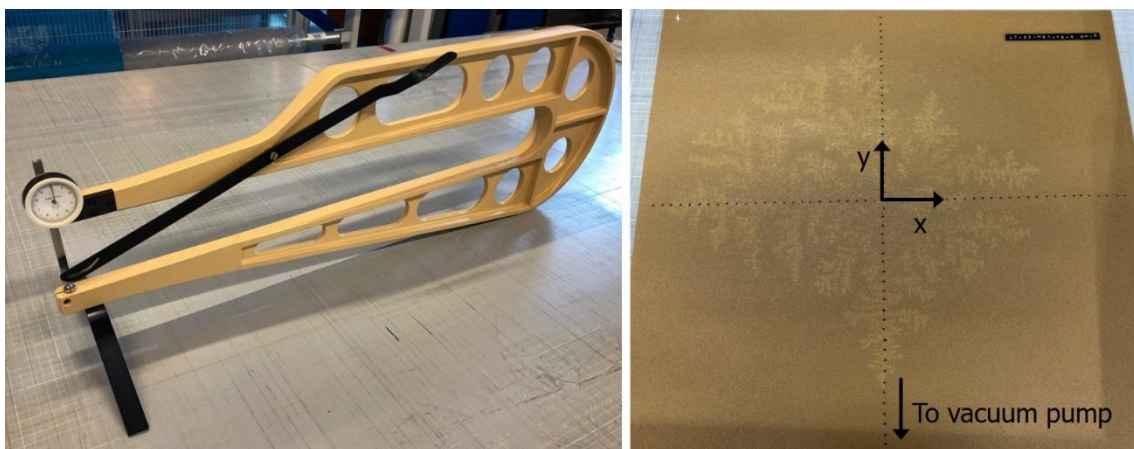
Figure 8: Thickness gauge and test grid on a test plate with the leakage at the origin
