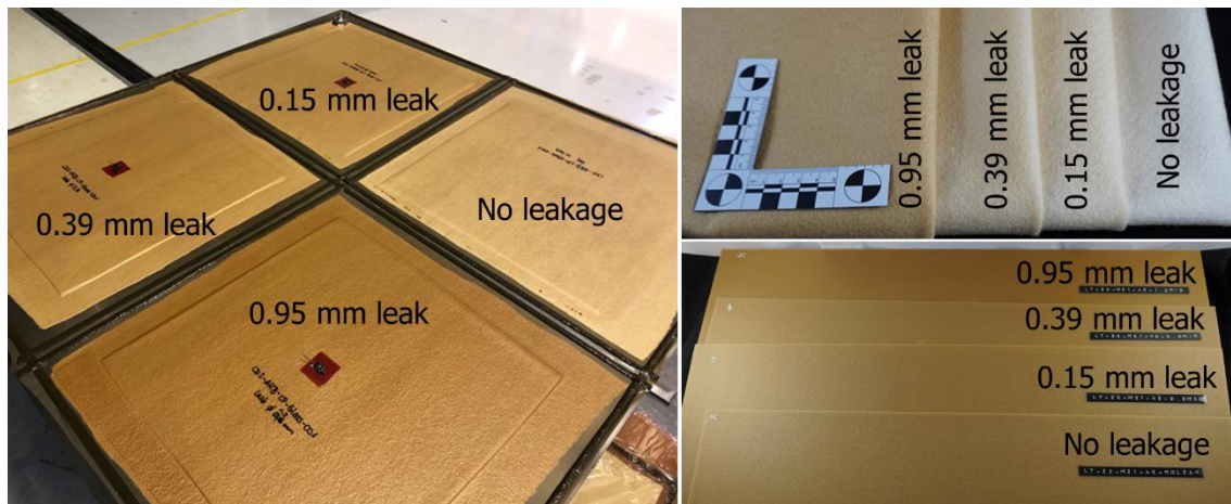
Figure 10: Colour gradation of vacuum bags, breather and laminate right after autoclave cycle
