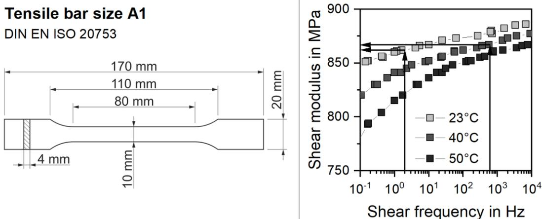
Figure 7: Tensile bar (left) and shear frequency dependent modulus (right)
