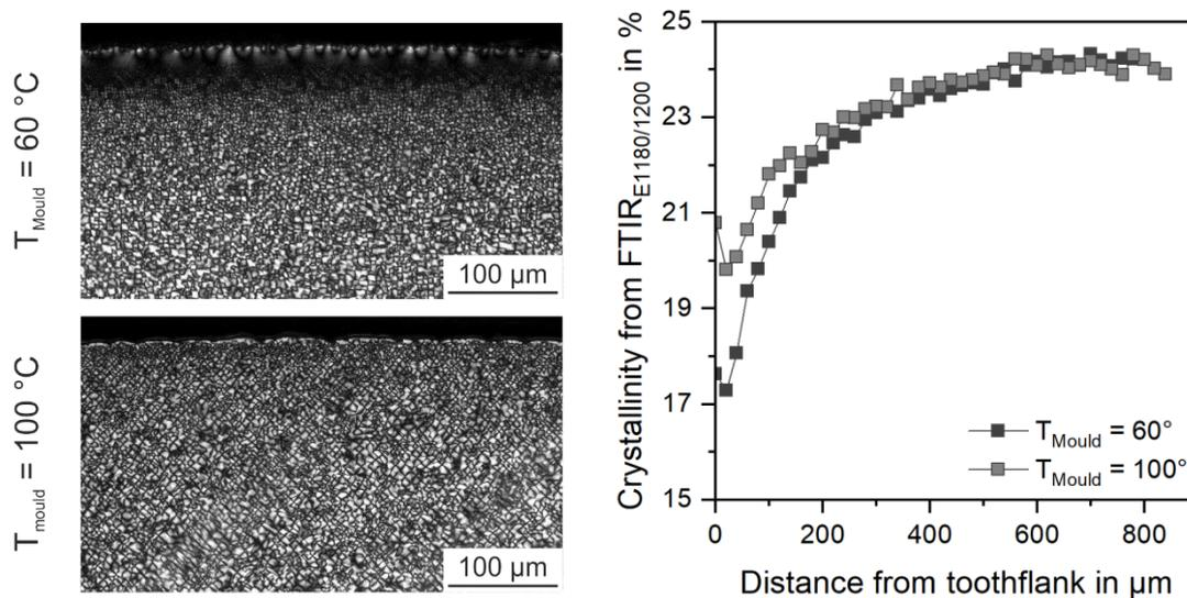
Figure 10: Morphological differences due to mould temperature
