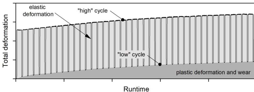
Figure 3: Distinction between elastic and plastic deformation and wear
