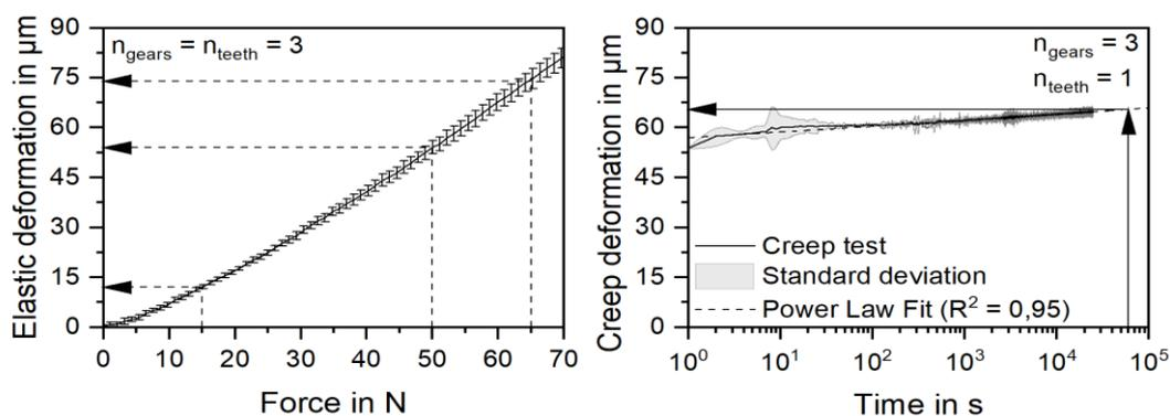
Figure 5: Elastic deformation (left) and creep (right) in the pulser test rig
