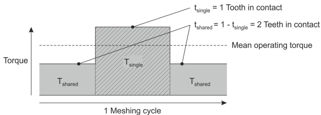
Figure 6: Simplified schematic of load sharing during the meshing cycle
