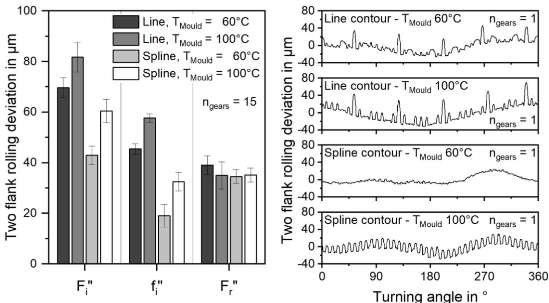
Figure 9: Two flank rolling deviations of the different specimens
