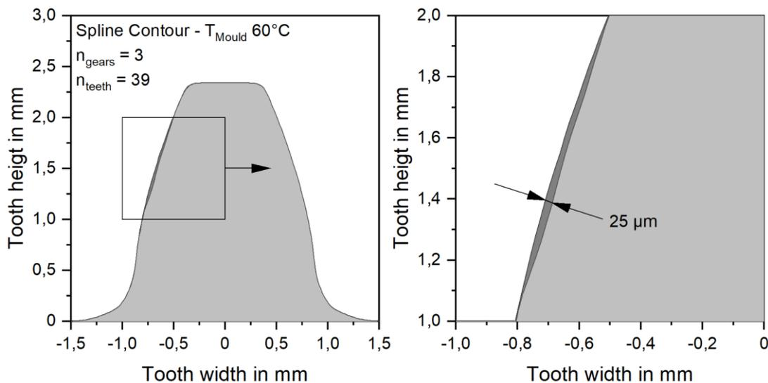
Figure 8: Mean tooth contours determined by coordinate measurement
