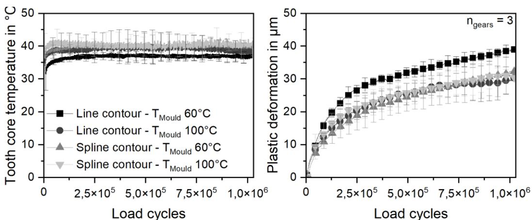
Figure 12: Influence of deviations on tooth temperature and plastic deformation
