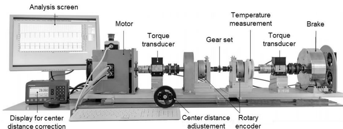
Figure 1: Main components of the in situ gear test rig
