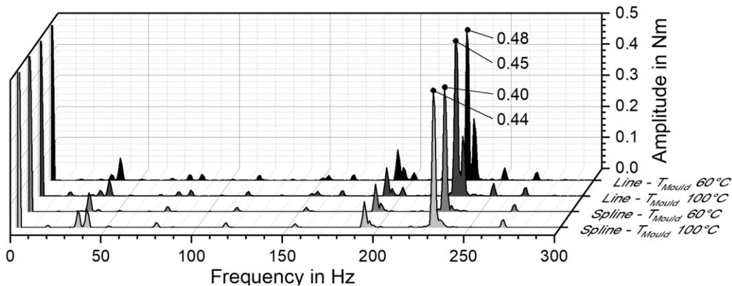
Figure 11: Influence of form and structural deviations on input torque variations
