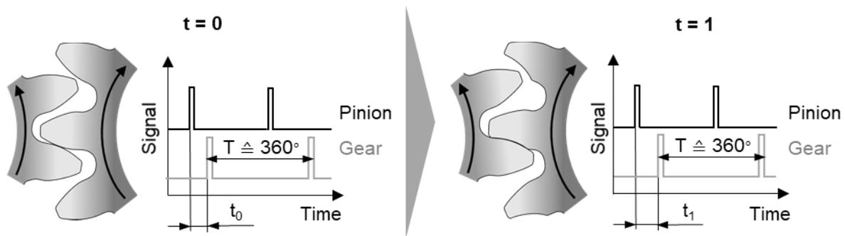
Figure 2: Tooth deformation induced angular displacement between input and output shaft
