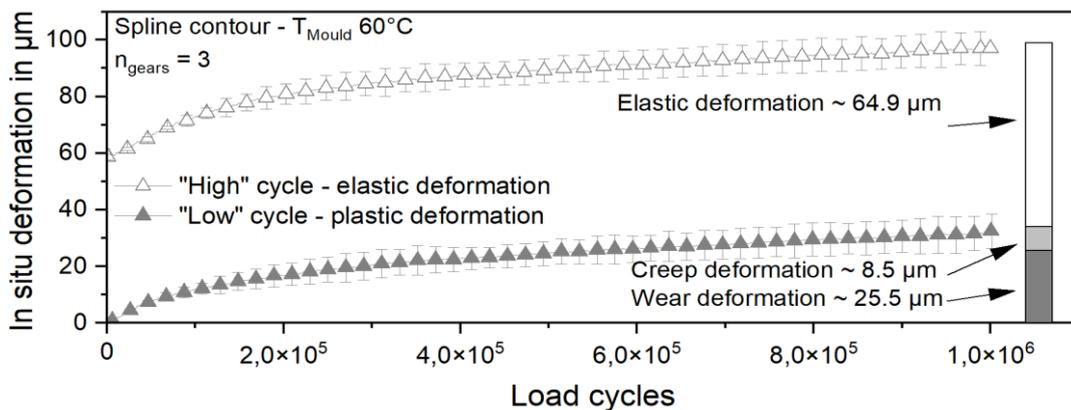
Figure 4: Correspondence of in situ and ex situ measurements
