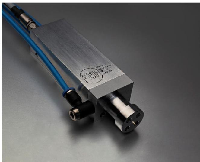
*Figure 1: Compact  $\mu$ -wave atmospheric pressure plasma device, developed by the Ferdinand-Braun-Institut, the plasma jet is visible as a small plasma flame at the front-side of the source*
