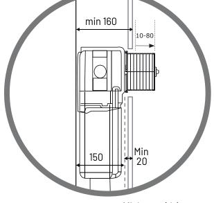
Minimum thickness from front of cistern to the front face of wall to be at least 20mm
