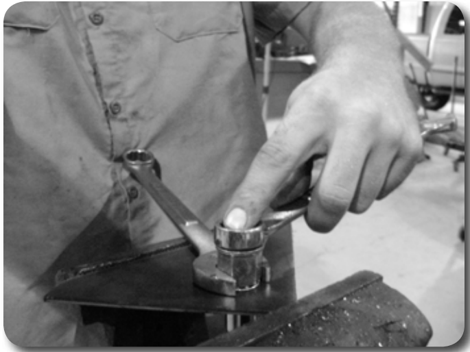
Figure 4 - 1/2" Rivet Nut shown
