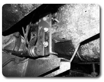
33. Install bracket as shown with factory nut at top mounting point – Fig 10.
