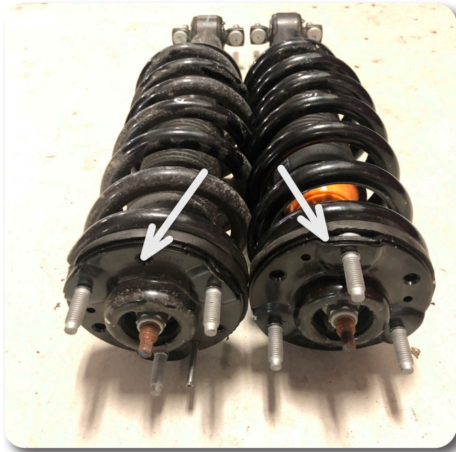
Figure 18 (Strut on the right has the top hat rotated 180 degrees, strut on the left is stock orientation with the bar pin angle the same)
