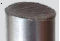
Image of the face of a 1/2" aluminum rod after 30 second of grinding using 40G alugrind Flap Disc.
