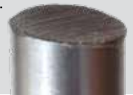
Image of the face of a 1/2" aluminum rod after 30 second of grinding using 40G alugrind Flap Disc.
