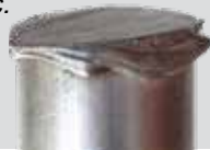
Image of the face of a 1/2" aluminum rod after 30 second of grinding using 40G Ceramic Flap Disc.
