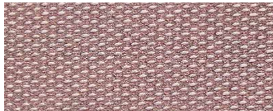
Image of the face of a 1/2" aluminum rod after 30 second of grinding using 40G Ceramic Flap Disc.
