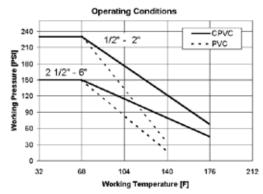
Pressure temperature rating for water. Socket fusion only. Threaded and flanged have a 10 bar (150 psi) maximum rating.
