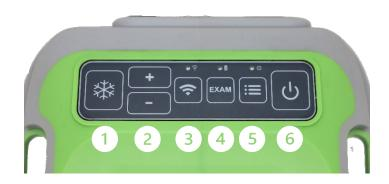
**5 - Menu**: Pressing this button will bring up the right menu, which allows you to adjust image settings like gain, dynamic, frequency, etc. Use the exam button to scroll through the menu, and the +/- buttons to adjust the settings. Press the menu button a second time to bring up the left menu which will allow you to adjust your grid, wireless channel, etc. Press the menu button a third time to exit the menu screen. See more videos online for settings help.
