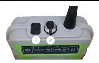
1 – Charging Port: The charging port is on the top of the ultrasound, all the way on the left. Lift the flap from the front of the machine to expose the charging port. Keep the flap closed and sealed when not charging the ultrasound to keep water, dust, and debris out of the charging port. Light above the exam button (#4) blinks when charging and is solid when charged. Only use chargers provided by ReproScan to charge your ultrasound!
