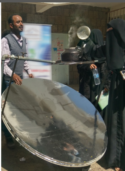
Course participants show how the foil-covered satellite dish of their simple solar cooker reflects the heat of the sun onto the cooking pot suspended above it. Photo: Tearfund's partner
