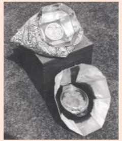
the tin outwards, above the ruler, till they are like the petals of a flower (**3**). Cut out corner pieces (**4**) which have sides the same length as the 'petals', allowing a small overlap. Using this overlap, attach the pieces to the 'petals' with nuts and bolts or rivets (**5**).
