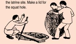
**5** You can use the slab over a 1.1m diameter unlined pit, but there is a danger that the sides might collapse, so it is better to have a pit with a lining at the top to match the diameter of the slab.
