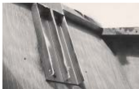
The metal vent at the back allows hot air to exit the drier.
