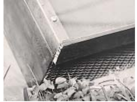
Hot air enters via the front vent and is drawn up through the drier.
