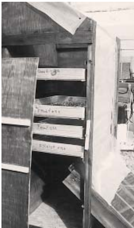
View of the drier with side removed, showing arrangement of inlet and trays.
