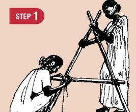
Tie the poles very tightly together to make the shape of a letter A. Hang the stone from the top of the A-frame, making sure the stone hangs below the cross bar.
