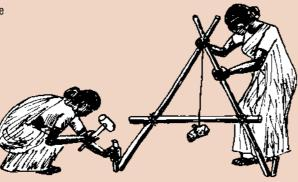
This will result in a line of small sticks. Smooth out any sharp bends in the line and use this line as the guide for building bunds and contour mounds.
