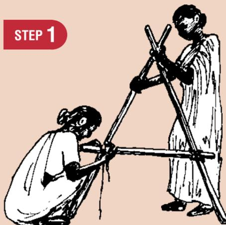
Tie the poles very tightly together to make the shape of a letter A. Hang the stone from the top of the A-frame, making sure the stone hangs below the cross bar.
