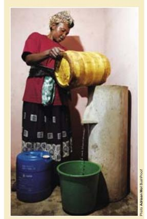
Water is poured slowly into the filter and safe filtered water is collected from the spout.
