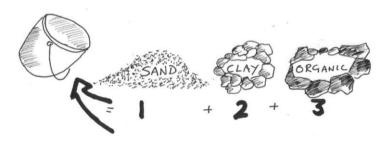
A typical soil quality test is to roll a small lump of soil in your hand. If it holds its shape when rolled, but snaps when bent, it should be suitable. Soil that crumbles contains too much sand. Soil that doesn't easily break contains too much clay.
