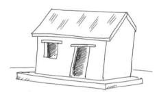
Could houses be built on raised plinths made from soil, a little cement and some pieces of stone and brick? These can be built strong and high enough to last through repeated floods, unlike traditional earthen floors that simply wash awav.
