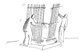
Could lightweight walls be built? In warm climates, bamboo and jute (or local equivalents) can make resilient walls that cost very little, are quick and easy to replace, and can be dismantled and carried to high ground if people receive warning of a major flood.
