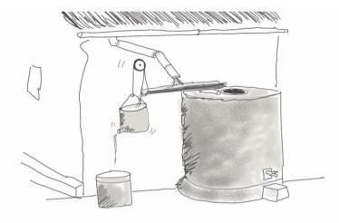
There are different ways of creating a first-flush diversion system. The simplest method is to move the downpipe at the start of a rain episode so that the water spills onto the ground rather than going into the tank. However, this relies on somebody being at home when the rains start, and that they remember and are prepared to go out into the rain to operate it! Other methods do not rely on somebody operating them. Here are two examples:
