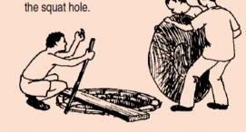
You can use the slab over a 1.1m diameter unlined pit, but there is a danger that the sides might collapse, so it is better to have a pit with a lining at the top to match the diameter of the slab.
