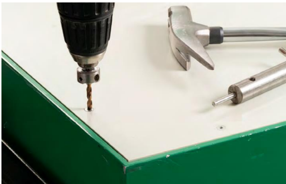
Figure 19: Remove rivet head (drill out)
