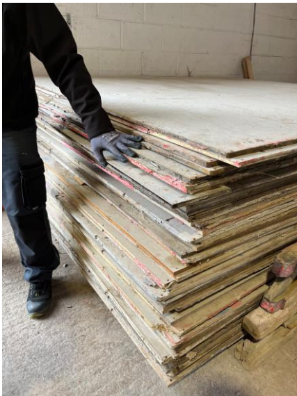
Figure 17: Replaced panels (plywood)
