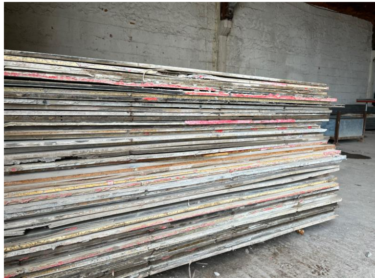
Figure 18: Waste generation from replaced panels (plywood)
